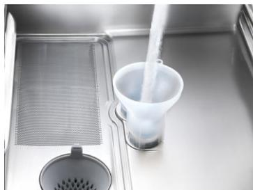
Place the funnel in the filling opening on the salt container and gradually add 3 bags of Winterhalter special salt (=1.5 kg). Remove the funnel and clean any salt residue from the filling area.
