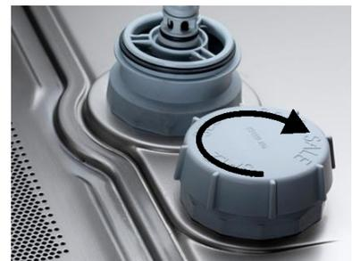
Screw the salt container tight again, keeping the cover straight. Re-install the bottom rotating wash field. Check whether the wash field rotates easily.
